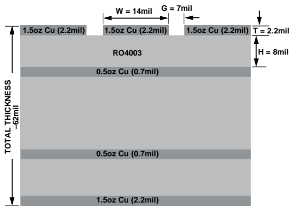
Figure 23. Evaluation Board Cross Sectional View
