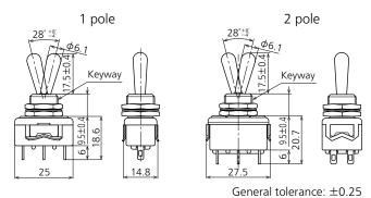
Note) ON-OFF type does not have terminal No. 1 and 4.
