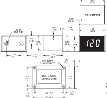
$\begin{array}{ll} \mbox{Dimensions in inches (millimeters)} \\ \mbox{Tolerances:} & 2 \mbox{ PL Dec } \pm 0.02 \ (\pm 0.51) \\ \mbox{ } 3 \mbox{ PL Dec } \pm 0.010 \ (\pm 0.254) \\ \mbox{Recommended panel cutout dimensions:} \\ \mbox{ } 1.336 \ (33.93) \mbox{W} \times 0.838 \ (21.29) \mbox{H} \\ \end{array}$
