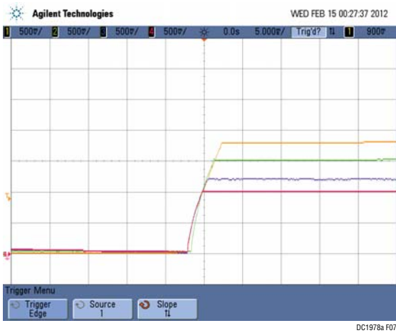
Figure 7. Tracking Supplies Up with DC1978A
