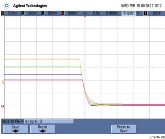
Figure 8. Tracking Supplies Down with DC1978A
