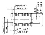
Recommended metal mask pattern Metal mask thickness: When 150 μm (Terminal opening ratio: 48%) (Metal-part opening ratio: 100%)
