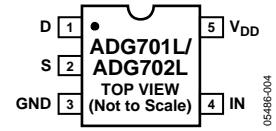
Figure 5. 5-Lead SOT-23 Pin Configuration
