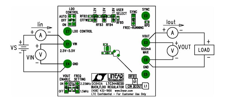
Figure 1. Proper Measurement Equipment Setup
