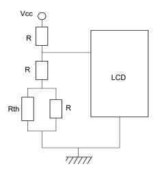
Temperature compensation (RF circuit)
