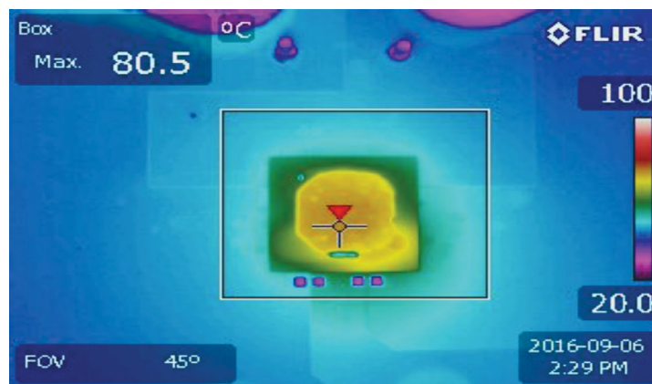
Figure 4. Thermal Image, V_{IN} = 12V , V_{OUT} = 1.0V , I_{LOAD} = 40A , Ambient Temperature = 23.0^{\circ}C , No Forced Airflow
