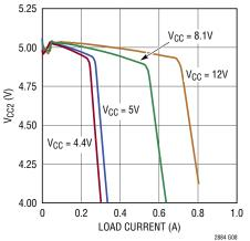
Derating for 125°C Maximum Internal Operating Temperature
