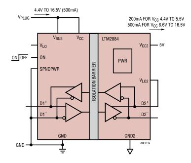
Figure 12. Isolated 1W or 2.5W Power Supply
