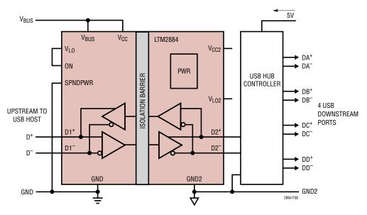
Figure 8. USB Hub Upstream Isolator
