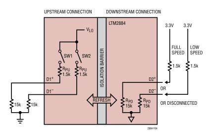
Figure 4. Idle State Automatic Resistor Setting
