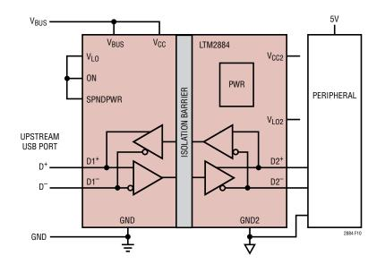
Figure 10. Powered Peripheral Device with USB Isolation and Low Current Suspend
