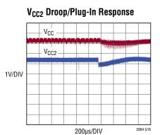
Upstream V<sub>BUS</sub> Droop During Plug-In with  $C_{LOAD} = 100 \mu F$
