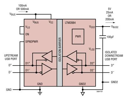
Figure 7. Bus Powered Inline Bus Splitter
