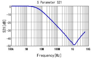
NFM15CC222D1A3 S21 DCOV, 25degC, Feedthrough
