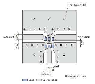
Line width should be designed to match  $50\Omega$  characteristic impedance, depending on PCB material and thickness.
