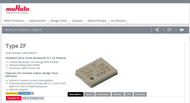
Type ZF BLE module supports Bluetooth 4.1 LE standard. All protocol stacks required for Bluetooth low energy communication are built in, including various healthcare profiles.
