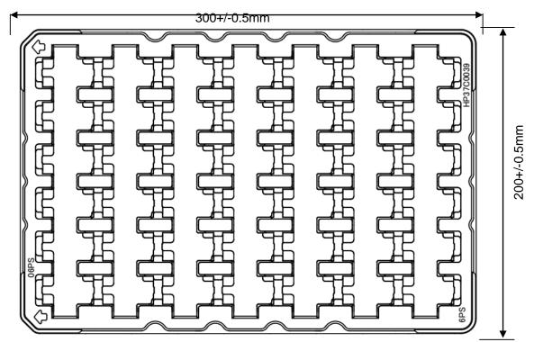
The module is placed in a pocket of the above tray with following rules.
