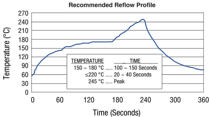
**Do not expose the breaker to temperatures exceeding +260 °C.**
