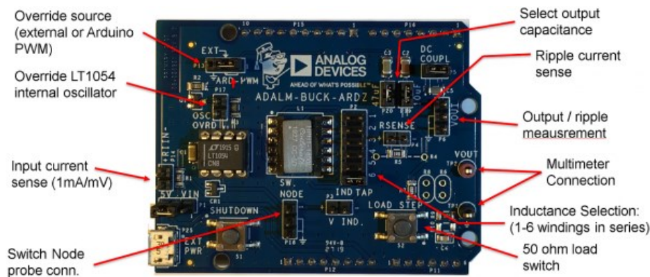
Figure 1. ADALM-BUCK connections and jumpers
