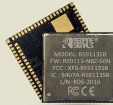
Module without integrated antenna
