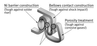
V notch and Double contact constructions
