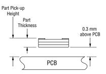
Recommended pick-up height: The bottom of the device should be 0.3 mm above the PCB.
