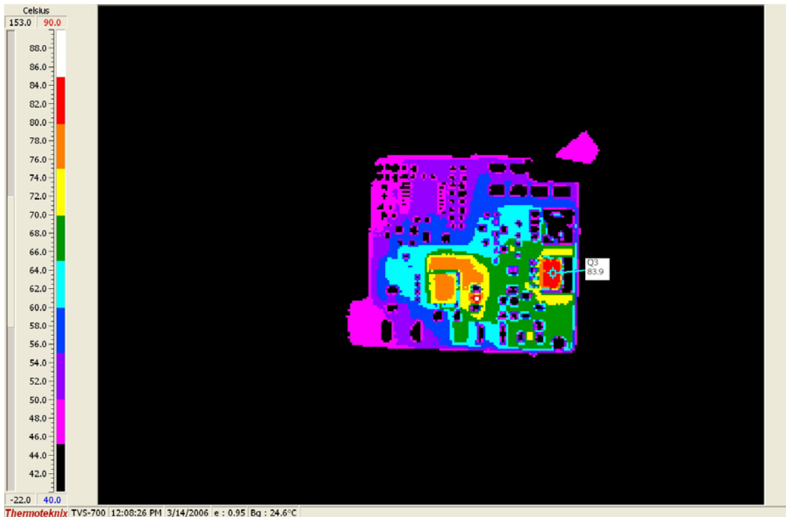
Figure 8. Temp Data (48Vin, 8A, 100LFM airflow – back)
