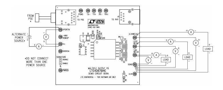
Figure 1. Proper Measurement Equipment Setup
