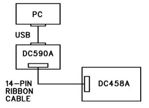
Figure 2. QuickEval Setup
