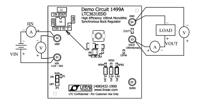
Figure 2. Equipment setup to test LTC3631
