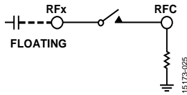
Figure 56. Series Capacitor Directly Connected to MEMS Switch
