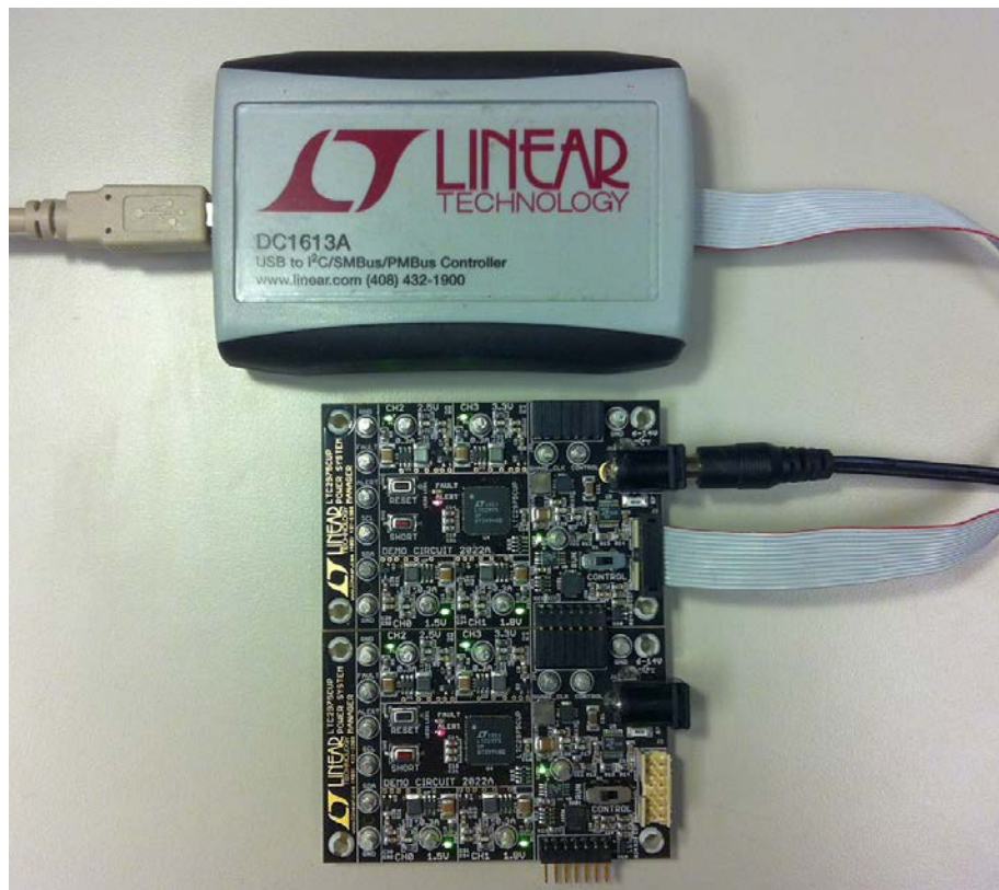
Figure 11. Array of Multiple DC2022A Demo Boards
