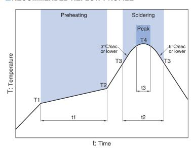
Soldering Preheating Critical zone (T3 to T4) Peak Temp. Time Temp. Time Temp. Time T1 T2 ТЗ **T4** t3\* t1 t2 60 to 120sec 150°C 200°C 217°C 60 to 120sec 240 to 260°C 30sec max.
