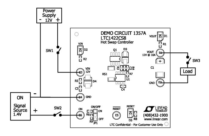
Figure 1. Proper Measurement Equipment Setup
