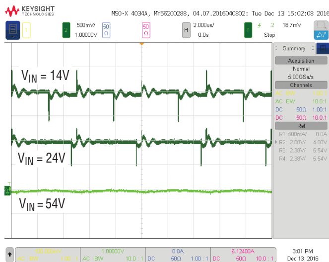
Figure 3. Output Voltage Ripple at 5A Output Current, V_{OUT} = 24V , 25MHz Bandwidth
