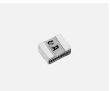
When using chip components in the design of FM radios, their arrangement and space allocation can create design difficulties. To help reduce these problems, Murata has developed this series of chip ceramic discriminators. They have heat resistant structures and allow the design of FM detecting circuits requiring no adjustment. Also, these discriminators yield stable demodulation characteristics. The CDACV10.7 Series can be used as kits with the Cerafil® SFECV10.7 Series to facilitate design.
