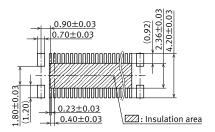
Recommended metal mask pattern Metal mask thickness: When 150 μm (Terminal opening ratio: 48%) (Metal-part opening ratio: 100%)
