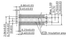
Recommended metal mask pattern Metal mask thickness: When 150 μm (Terminal opening ratio: 48%) (Metal-part opening ratio: 100%)
