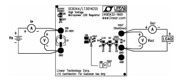
Figure 1. Proper Measurement Equipment Setup
