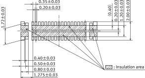
Recommended metal mask pattern Metal mask thickness: When 100 µm (Terminal opening ratio: 70%) (Metal-part opening ratio: 100%)
