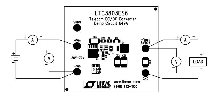
Figure 1. Proper Measurement Equipment Setup
