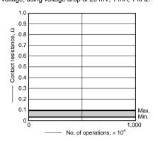
2-(2). Change in dynamic contact resistance (10 µA 1 mV DC resistive load) Tested sample: ASX20012, 10 pcs.
