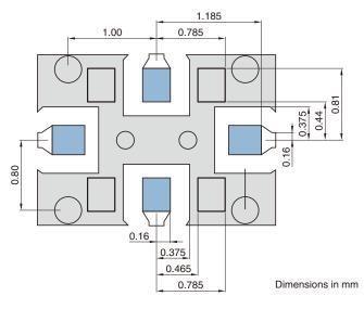
Line width should be designed to match  $50\Omega$  characteristic impedance, depending on PCB material and thickness.
