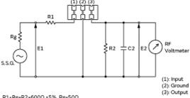
R1+Rg=R2=600Ω ±5%, Rg=50Ω C2=10pF (Including stray capacitance and Input capacitance of RF Voltmeter) E1: S.S.G. Output voltage
