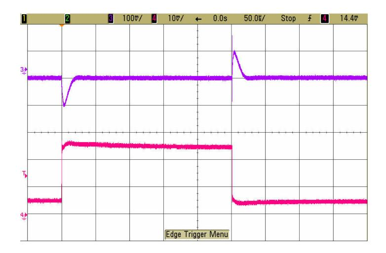
Figure 4. Load Step Response  $V_{IN} = 8.4V, V_{OUT} = 3.3V, 2A \text{ Load Step } (500\text{mA} <-> 2.5A)$  Forced Continuous Mode, Fsw = 1 MHz Trace 3: Output Voltage (100mV/div AC) Trace 4: Output Current (1A/div)
