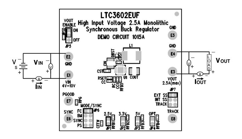
Figure 1. Proper Equipment Measurement Set-Up
