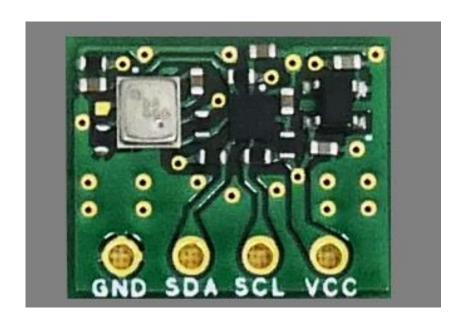
Barometric Pressure sensor device is capacitive type MEMS device combined with ASIC with I2C interface. Since its voltage level is 1.8V, there's level converter on this board, which enables user to connect directly to 3.3V system.
