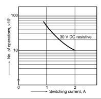
4. Mechanical life Tested sample: TK1-12V, 8 pcs. Switching frequency: 30 Hz
