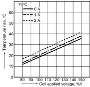
Measured portion: Inside the coil Ambient temperature: 70°C 158°F
