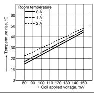
6.-(2) Coil temperature rise Tested sample: TK1-12V, 6 pcs.
