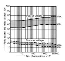
5. Electrical life (DC load) Tested sample: TK1-12V, 10 pcs. Condition: 2 A 30 V DC resistive load, 20 cpm Change of pick-up and drop-out voltage
