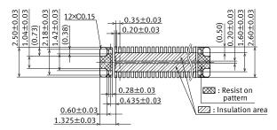
Recommended metal mask pattern Metal mask thickness: When 100 μm (Terminal opening ratio: 70%) (Metal-part opening ratio: 46%)
