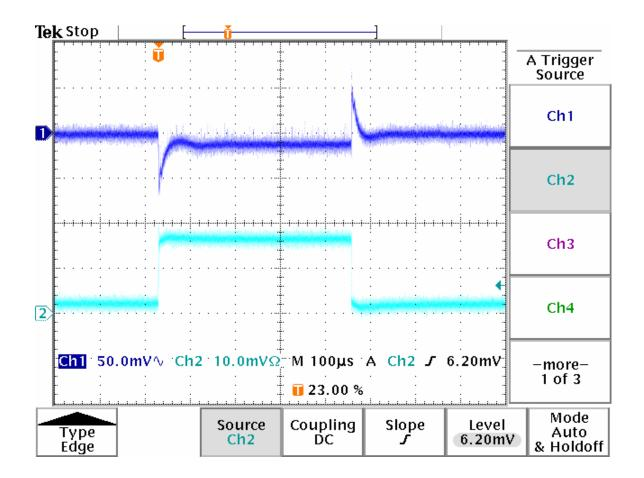
Figure 3. Load Step Response
