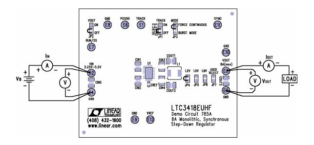
Figure 1. Proper Measurement Equipment Setup
