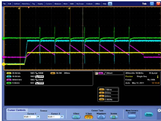
Figure 12. Power-Up into a Fault (TIMER); Channel 1 = VIN (Yellow); Channel 2 = V DS (Blue); Channel 3 = TIMER (Pink); Channel 4 = System Current (Green)
