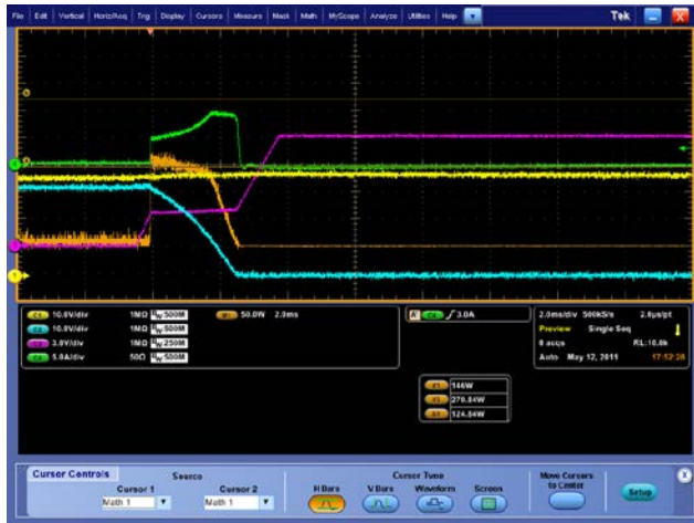
Figure 11. Power-Up Profile; Channel 1 = VIN (Yellow); Channel 2 = V DS (Blue); Channel 3 = Gate (Pink); Channel 4 = System Current (Green); M1 = FET Power (CH2 × CH4) (Orange)
