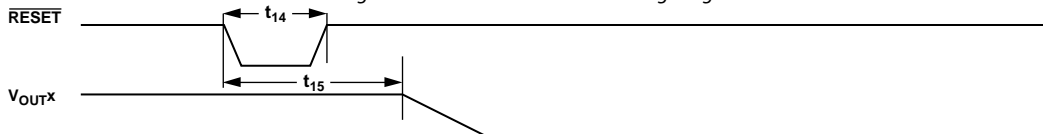
Figure 3. RESET Timing Diagram
