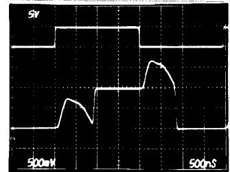
MUX-24 SMALL-SIGNAL SWITCHING WITH 2μs SAMPLE TIME
