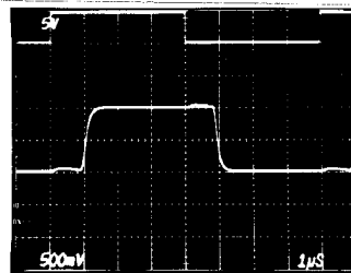
MUX-24 SMALL-SIGNAL SWITCHING WITH FILTERING
