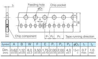
• Pitch 4 mm (Punched Carrier Taping) : Size 0603
