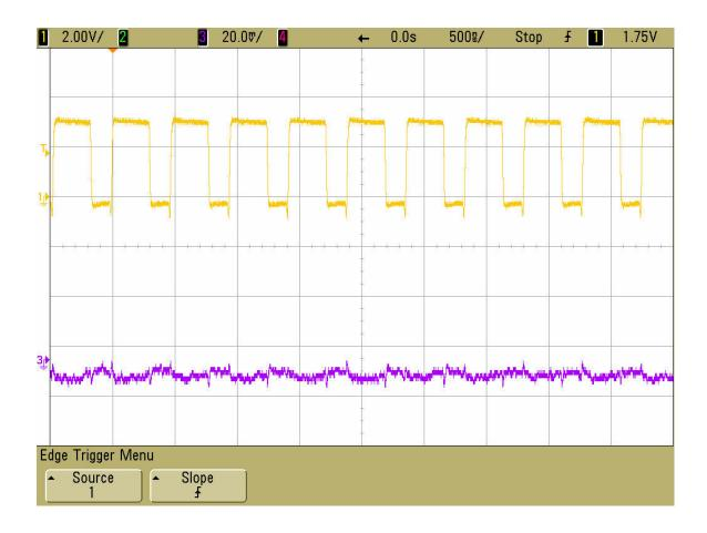
Figure 3. Switch Waveform & Output Ripple Voltage  $V_{IN} = 3.3V$ ,  $V_{OUT} = 1.8V$ ,  $I_{OUT} = 800mA$ Trace 1: Switch Voltage (2 V/div) Trace 3: Output Ripple Voltage (20 mV/div AC)
