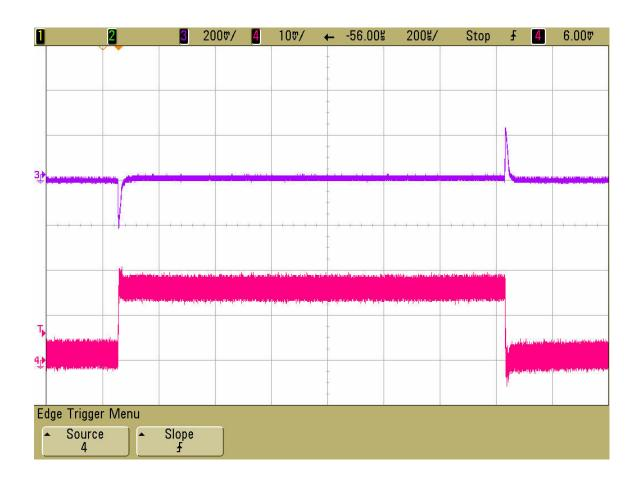
Figure 4. Load Step Response  $V_{IN} = 3.3V, \ V_{OUT} = 1.8V, \ 720mA \ Load Step (80mA <-> 800mA)$  Trace 3: Output Voltage (200mV/div AC) Trace 4: Output Current (500 mA/div)
