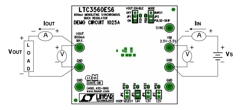
Figure 1. Proper Equipment Measurement Set-Up
