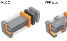
Internal electrodes are not conducting between terminal electrodes
