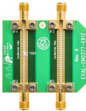
Figure 5. Calibration Transmission Lines
