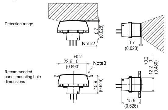
Note1: In order to ensure proper detection, install it with the lens exposed at least 6.2mm.(0.244inch) Note2: In order to ensure proper detection, install it with the lens exposed at least 0.7mm.(0.028inch)
