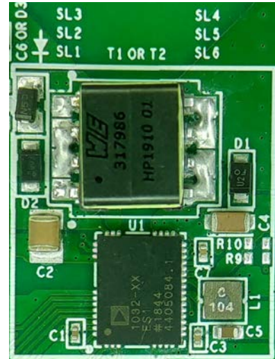
Figure 11. Solder Link Connections when Using T1
